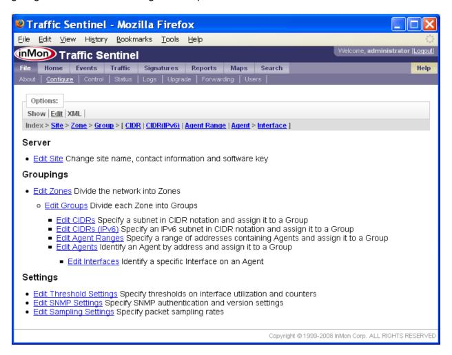
Traffic Sentinel uses SNMP to configure sFlow monitoring on HP ProCurve switches. Traffic Sentinel can be configured to automatically discover and configure sFlow provided that it is given the read-write SNMP community string and has "manager" privileges on the switch.
