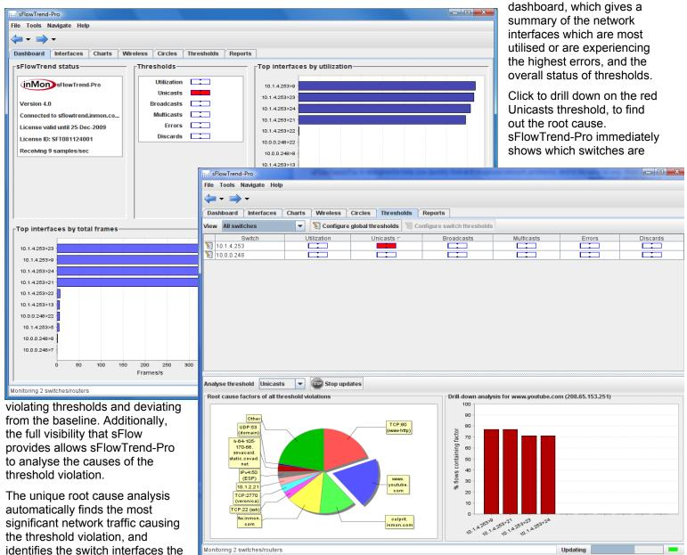
the traffic carried by a specific switch or interface can be viewed, to help determine if the traffic is normal, or if it is caused by a problem or network misuse. The traffic charts allow the history of traffic on an interface to be viewed (up to one week is retained by default), and to quickly determine if further action is required.
